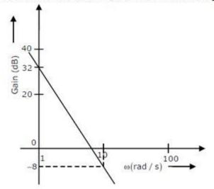
The gain (20 log G(s)) is 32 dB and -8 dB at 1 rad /s and 10 rad /s respectively. The phase is negative for all w. The G(s) is
